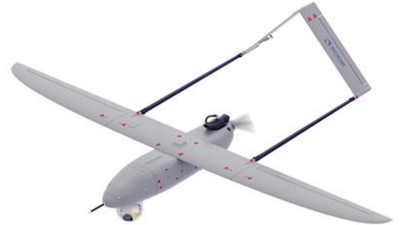
25 Hours Flight, 180km Range Long Endurance Unmanned Aircraft System.
