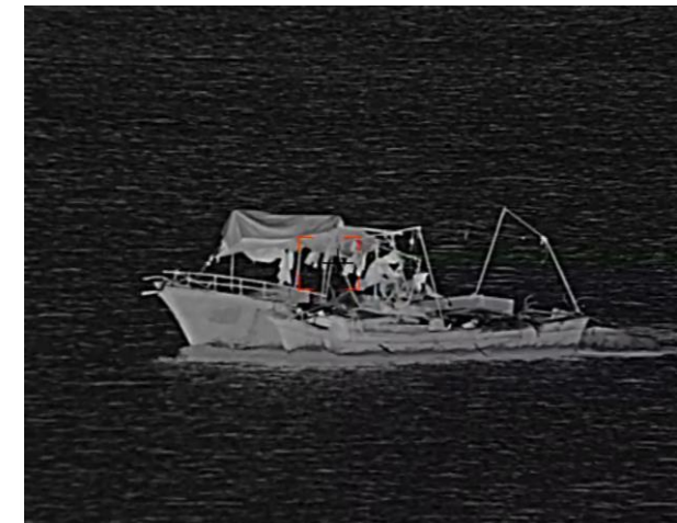
LWIR Uncooled Thermal Camera at 15Km.
