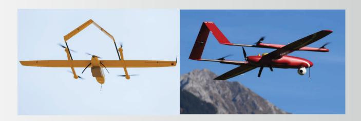
The ST-2H100 VTOL platform is made entirely of composite materials, which allows for exceptional strength and low weight, which is extremely important in the air. Since our designers come from aviation, they have transferred all the latest innovations in aerodynamics and aircraft construction to our UAV.
